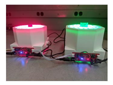
Each digital driver is based around an ATtiny85 microcontroller acting as an I2C peripheral. Multiple digital driver boards may be "networked" together onto one I2C bus by simply daisy-chaining the boards together, as shown above. In such a use-case you must choose a unique I2C address for each ATtiny85 peripheral.
