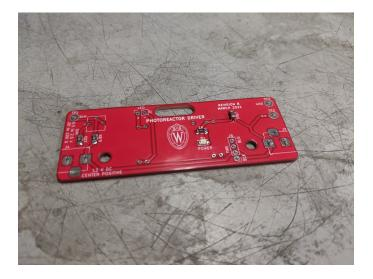
Begin by adding the surface mount components. Recommend thin solder, e.g. 0.015". The LED does have a polarity—ensure that the small green line points towards ground (left). Once done your board should look like the above.
