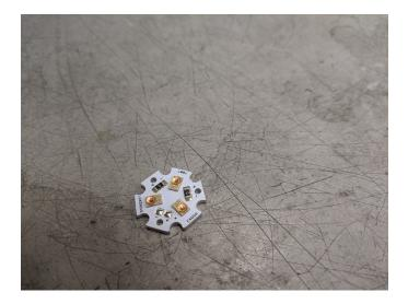
If possible, it's best to order your LEDs pre-attached to an "LED star" heat sink. Otherwise you may order bare LED stars and discrete LEDs. Either way, you will have a filled LED star as pictured above. In this example we are using LED Supply part number 07007-PL000-F.
