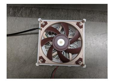
Install the fan. Pay special attention to the orientation of the fan, including the location of the cord. Use 3/4" screws here.
