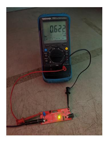
Next, add the barrel jacks and the test points. With these added you may plug in your board for the first time. You should see your power indicator LED illuminate. You should also be able to adjust the DC control voltage relative to ground by turning the knob, as shown above.
