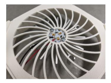
Install the LED star and heatsink with wires facing towards printed hole. Use 1/4" screws.
