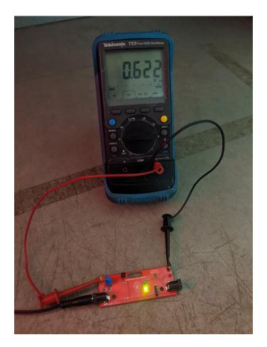
Next, add the barrel jacks and the test points. With these added you may plug in your board for the first time.
