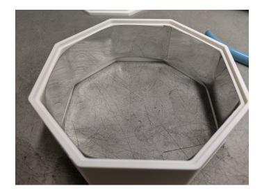
Simply cut the reflective material to line the chamber. It's good to leave overlap around the interior, as shown. Remove the backing and stick the material to the chamber walls.
