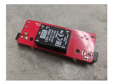
Finally, add the Mean Well LED driver. Note that this component goes on the back of the PCB, as shown above.
