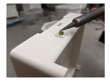
Each WPR base contains seven threaded heat inserts. These allow components such as the drive circuit board to rigidly attach to the base via machine screws. Use a soldering iron to carefully heat these while pushing them into their cavities.
