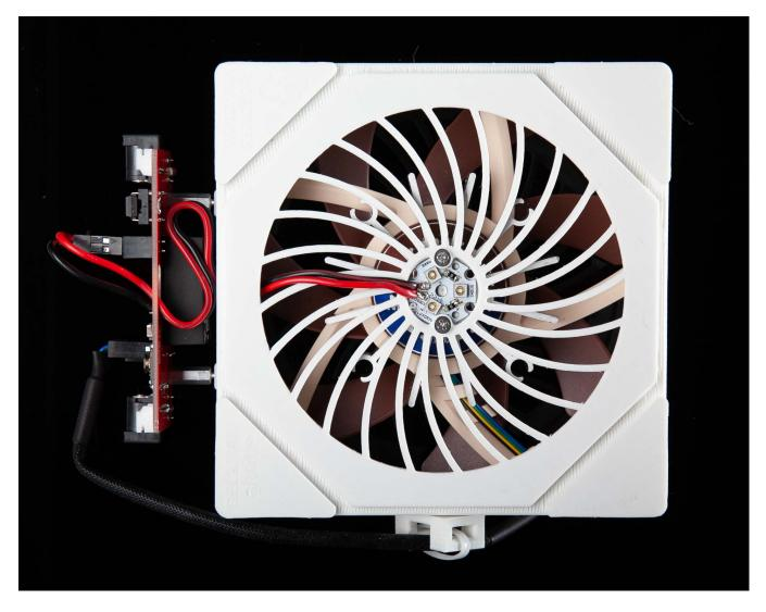
Once 3D printing is done and PCBs have been filled, WPR assembly is fairly straight-forward. The various electronic components must be installed into the base (pictured above), as described in subsubsection 2.4.1. Reflective coating must be added to the chamber walls, as described in subsubsection 2.4.2. After these final steps, your WPR is ready for synthesis!
