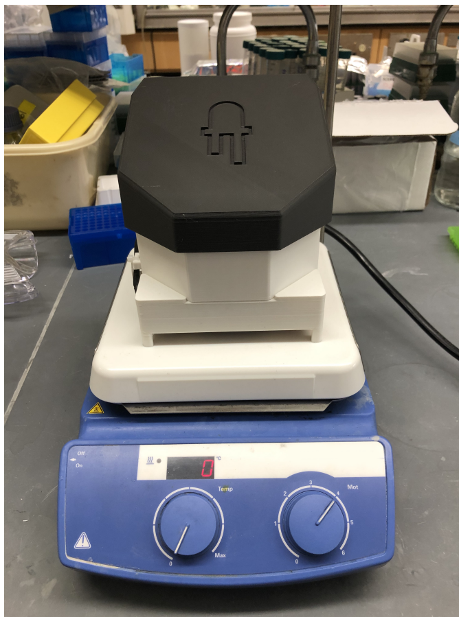
Figure 24: WPP device fitted the provided light shield cover module printed in black PLA.
