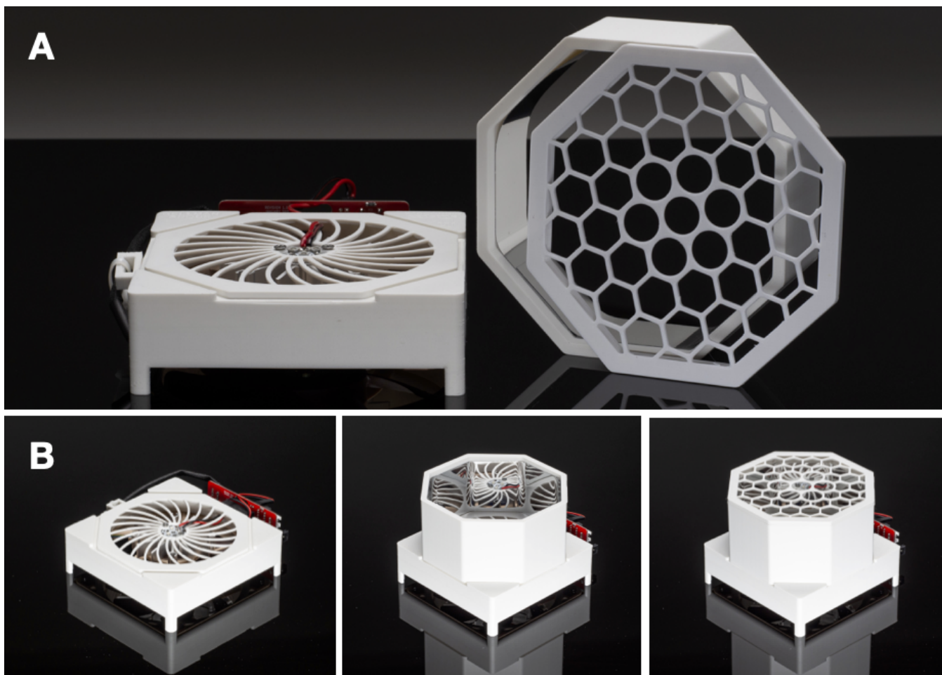
Figure 1: (A) Unassembled WPP device comprised of a vessel holder, reaction chamber and standardized base fitted with a digital driver board. (B) Modular apparatus assembly.
