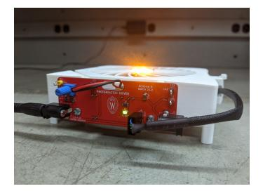
pins: blue: PWM (5 V) yellow: +12 V black: ground 0.5" standoff: RAF 4505-440-AL TODO: LED PINS SOLUTION
