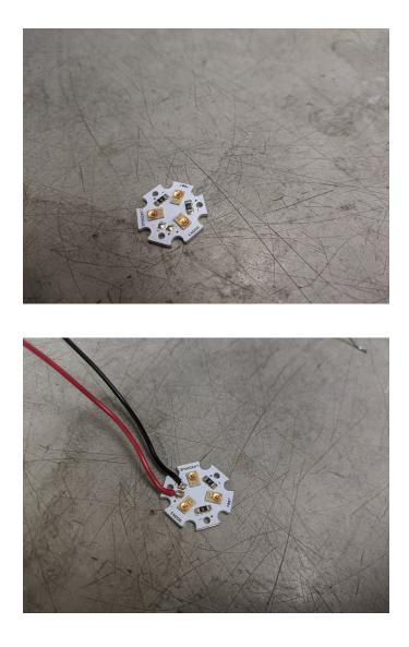
In this case LED Supply 07007-PL000-F May be a challenge—heat sinking will fight you Add lead-based solder to make easier
