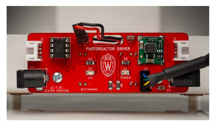
The WPR incorporates small circuit boards controlling the incorporated LED and fan. We refer to these small boards as "drivers". There are two types available: the "analog-driver" and "digital-driver". Refer to the associated directories in the online repository for design files for each of these.
